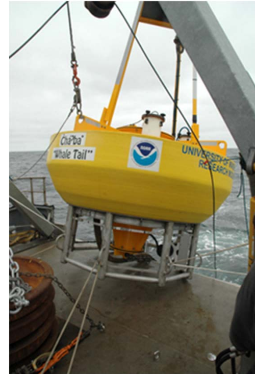
“Chá bă,” a new buoy off the coast of Washington, contributes better information about the ocean conditions that oysters can and cannot tolerate. (photo: J Payne, Pacific Ocean Shelf Tracking Project)
