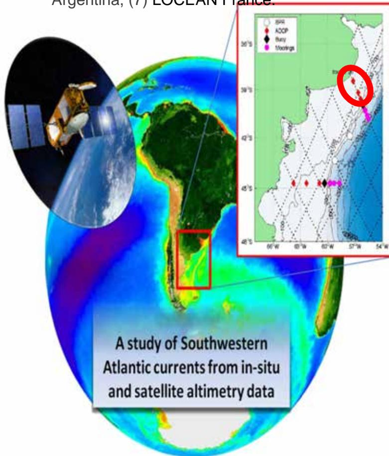
Altimetry products are compared with in situ time series of currents, T and S obtained in two moorings located under Jason track #26 at about 40°S. Each single correction applied to altimetry data to construct SLA is considered.
