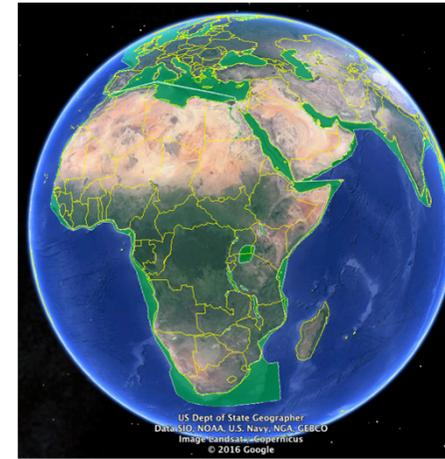
Actual **mode mask** for coastal and ocean areas (used to calculate the SAR data volume)
