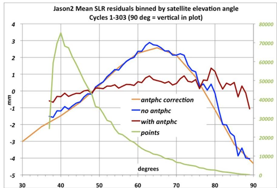
*Mean (& RMS) residuals show LRA phase center modeling IS improved with satellite elevation angle (antphc) correction (mm)*
