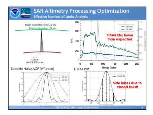
Despite the fact that the FF-SAR 2D point target response shows the expected ~0.5 meter resolution in the along-track and slant-range dimensions, the full along-track PTR shows side-lobes that are due to the lacunar sampling of the Doppler spectra, originated by the closed burst operation.
