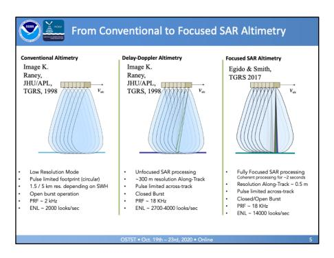
In this slide we put in perspective three different nadir looking processing techniques: the conventional pulse limited altimeter, the delay/Doppler processing, and the fully-focused SAR altimeter.
