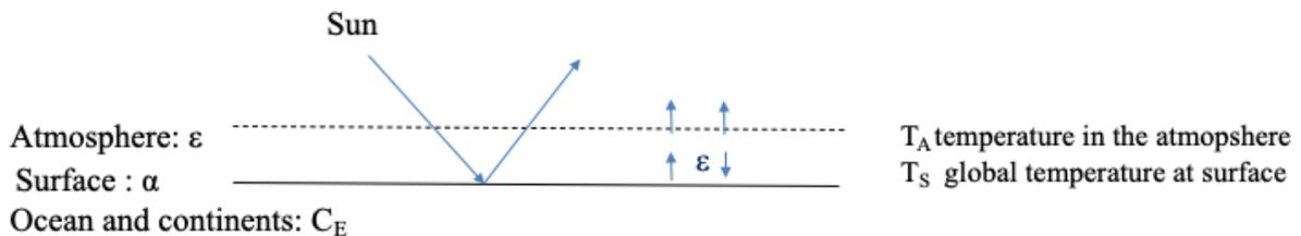
$$C_E \frac{\partial T_S}{\partial t} = \frac{S_0}{4} (1 - \alpha) + \epsilon \sigma T_A^4 + (1 - \epsilon) \sigma T_S^4$$
