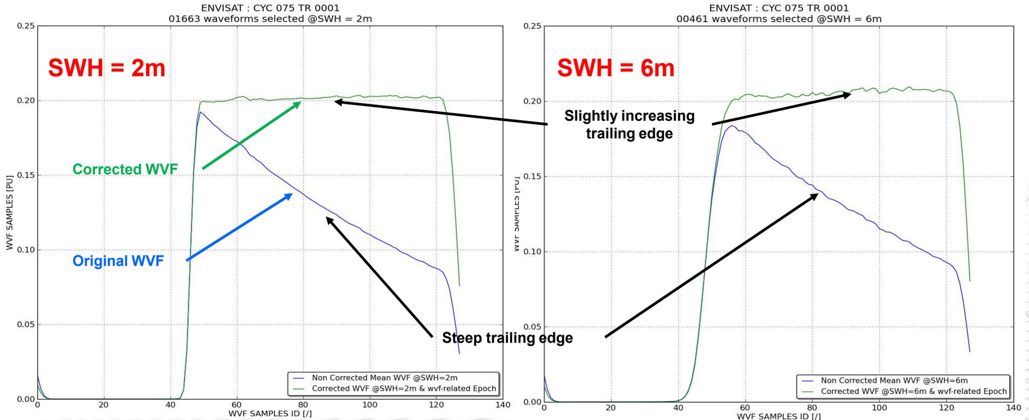
**Filter correction included in the RA-2 waveforms**
