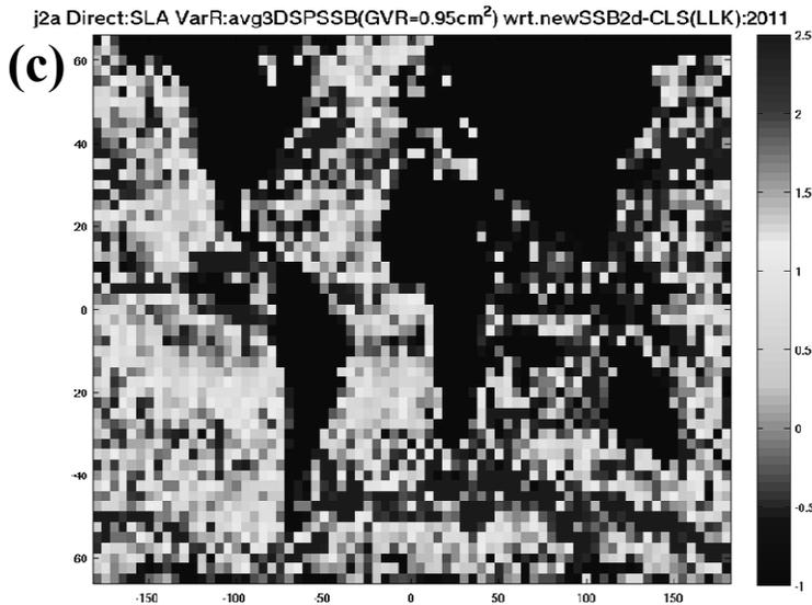
**J1a/J2a: Collinear difference test : Variance Reduction (positives indicate performance gain) varying with latitude, obtained using the 2D and 3D SSB models relative to a 2D CLSSSB**
