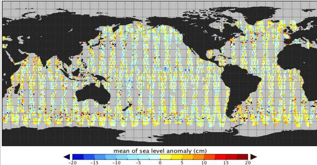
The Jason-2 orbit repeats every 10 days. One such 10-day period is shown here (J2 cycle 91). The areas sampled by CryoSat during 10 days move with each 10-day cycle. Differences are computed in  $1 \times 1^\circ$  boxes and then these boxes are area-weighted averaged to give the global mean sea level difference estimated every 10 days.
