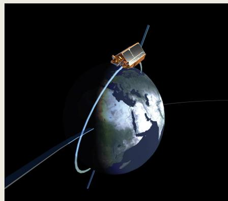
Because CryoSat is not sun-synchronous, its orbit plane makes a half revolution with respect to the Earth-Sun line in about 244 days. We can use it to explore the 59-day errors in TOPEX/Jason data.
