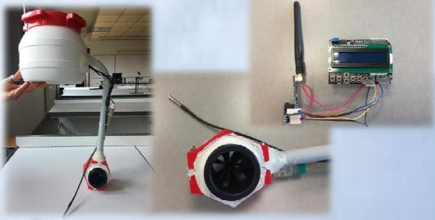
Creation and production of the 1<sup>st</sup> cylinder with different receivers (speed, temperature, pH) as well as a radio transceiver to receive and view data directly.
