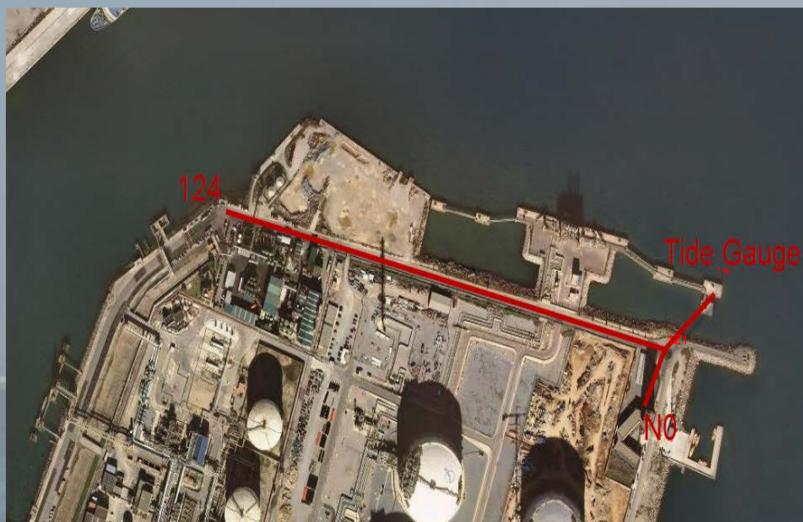
General view of the levelling traverse conducted in 2009 and repeated in September 2011 (red line, about 700 m along the northern side of the "Energy Pier", Barcelona harbour, Spain). The levelling chain links points #124 (Levelling Network XdA), the Tide Gauge (point #146) and the Harbour Control Tower (NO point is located at the ground floor of the Tower, whereas the GPS Station- ARP point- is at its roof). Source of the orthophotomap: Institut Cartogràfic i Geologic de Catalunya (ICGC).
