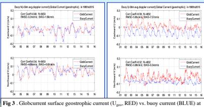
**Fig 3.** GlobCurrent surface geostrophic current ( $U_{geo}$ , RED) vs. buoy current (BLUE) at station N (left) and I (right). The upper lower panels show U and V current components.
