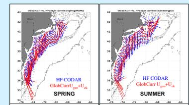
**Fig 6.** Comparisons of seasonal mean surface current vectors in HF Codar measurements (BLUE) and altimeter-based GlobCurrent  $U_{total} = U_{geo} + U_E$  (geostrophic) +  $U_E$  (Ekman) (RED). The 100-, 1000- and 4000-m isobaths are also shown.
