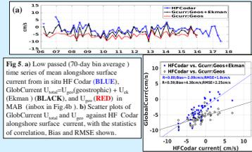
**Fig 5.** a) Low-passed (70-day bin average) time series of mean alongshore surface current from in situ HF Codar (BLUE), GlobCurrent  $U_{total} = U_{geo} + U_E$  (geostrophic) +  $U_E$  (Ekman) (BLACK), and  $U_{geo}$  (RED) in MAB (inset in Fig. 4b). b) Scatter plots of GlobCurrent  $U_{total}$  and  $U_{geo}$  against HF Codar alongshore surface current, with the statistics of correlation, Bias and RMSE shown.
