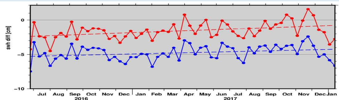
A drift in S3A SAR SWH of +1.12 cm/year translates in a drift in S3A SAR SSB of around -0.36 mm/year which is not a negligible error in the global mean sea level rise estimation.
