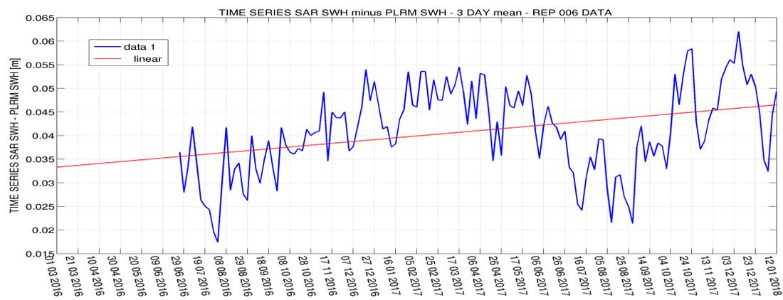
Furthermore, the S3A SAR SWH is drifting in time with respect ECMWF model by 1.12 cm/year and with respect to the Jason-3 mission, the drift of S3A SAR SWH is 1.03 cm/year.
