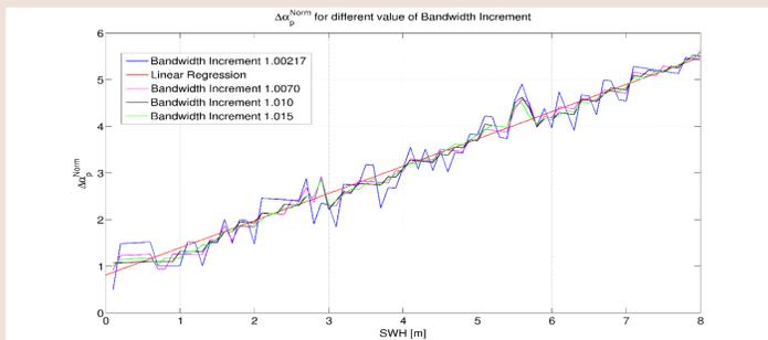
These numerical simulations have been repeated for various values of the PTR change factor in order to prove that the Equation (1) does not depend significantly on the used value of the change factor of the PTR width
