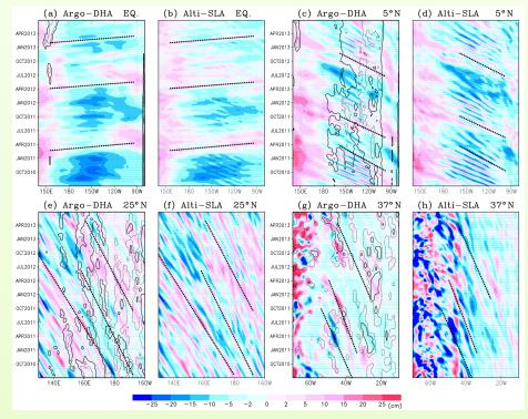
Fig.6 *x-t* diagrams of analyzed Argo DHA and altimeter SLA along four sections. DHA is SSDH (0-1200 dbar) anomaly from the monthly mean SSDH obtained from WOA2009. Refer Fig.7 for location of the sections.
