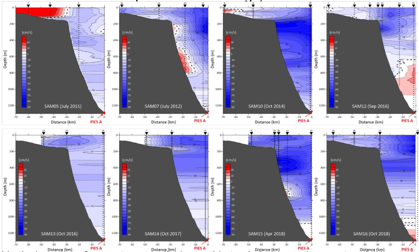
*Vertical section of current perpendicular to ship track, between the coast and 1<sup>st</sup> mooring of SAMBA array, between July 2011 and Oct. 2018 (SAM project, courtesy of D. Valla).*
