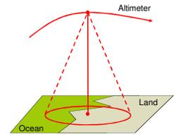
Figure 2a: DEM altitude selection in the altimeter footprint. As oceans have higher priority than land, the altitude assigned to the nadir point is the altitude of an ocean point.
