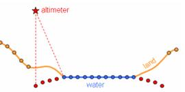
Figure 2b: Extension of an area of interest due to surface type priority (water) and slant view correction.
