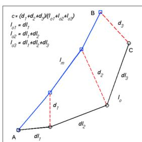
Figure 7: Diagram of skill score principle as proposed by Liu et al. Adapted from Liu and Weisberg, 2011.
