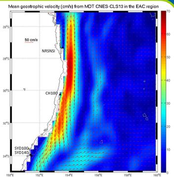
Figure 2: Mean geostrophic velocities derived from the CNES-CLS13 MDT off New South Wales (EAC in red) and ADCP stations.
