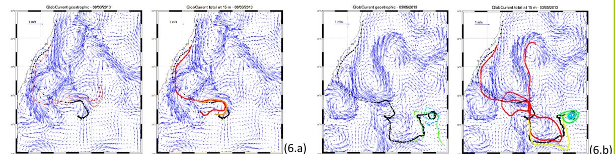
Figure 6: Snapshots ((a) and (b)) of trajectories over the time of pseudo-drifters (in colors) advected by the fields of GlobCurrent total surface currents at 15 m (right plot) or GlobCurrent geostrophic currents (left plot). The positions of the real drifter are in black. The GlobCurrent velocity fields used to advect the pseudo-drifters are shown with blue arrows.
