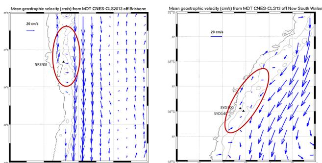
Figure 4: Mean geostrophic velocities from the CNES-CLS13 MDT off Brisbane (left) and off Sydney (right). Black triangles show the ADCP stations. The light-gray lines show the 100-m and 200-m isobaths.
