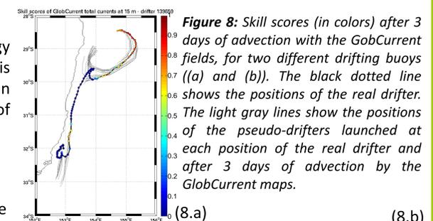
Figure 8: Skill scores (in colors) after 3 days of advection with the GobCurrent fields, for two different drifting buoys ((a) and (b)). The black dotted line shows the positions of the real drifter. The light gray lines show the positions of the pseudo-drifters launched at each position of the real drifter and after 3 days of advection by the GlobCurrent maps.
