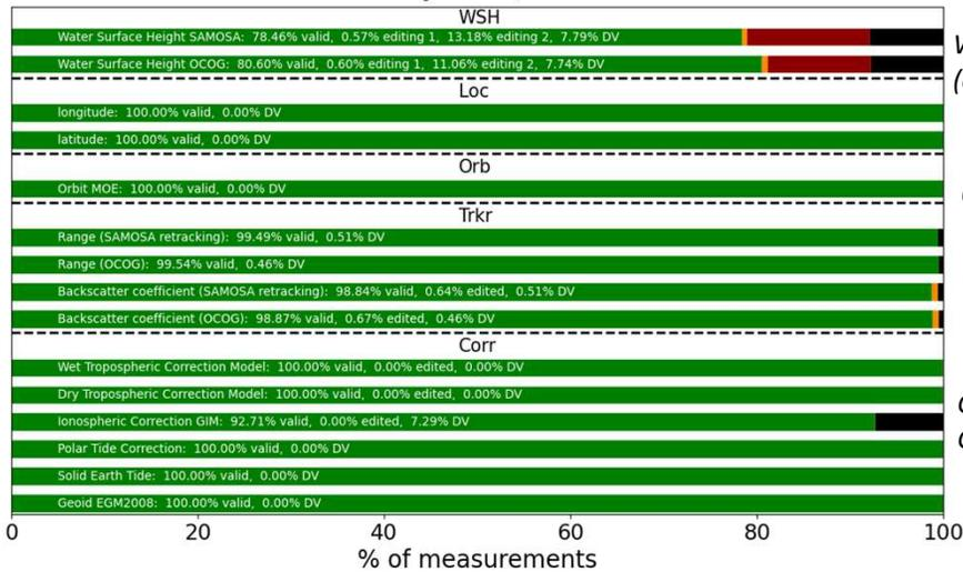
**METRIC** : Percentage of valid (green), erroneous (tests using boundary values condition : orange and red) and NaN data (black)
