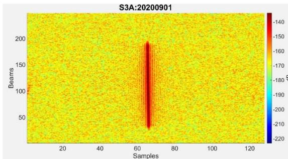
Fully Focused processed TRP signal from 1<sup>st</sup> of September 2020
