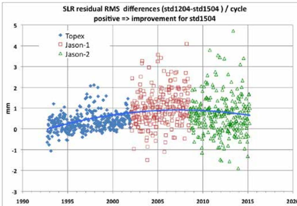
**Std1504 radial orbit accuracy relative to std1204 using SLR data.**
