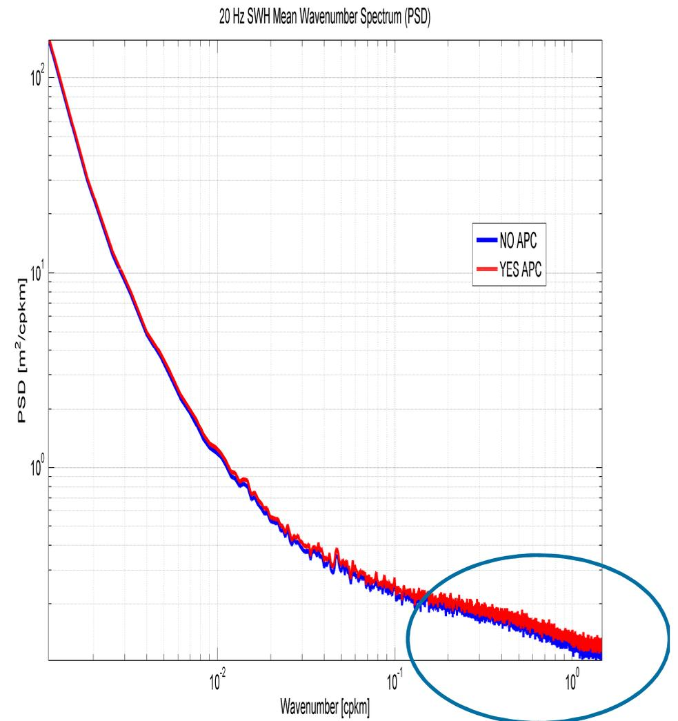
Wave Number SWH spectra with APC ON is **slightly degraded** (in term of spectral noise), no major anomaly from the dispersion density plot
