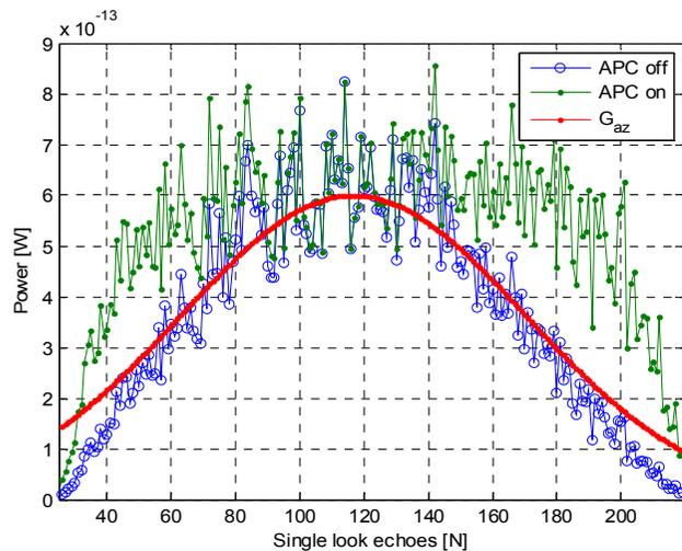
The speckle from all the single look echoes in the stack is raised approximately to the same power. A better speckle reduction is expected. In case APC is applied, Multilooked waveforms are built from  $\approx$  **180** Single Look Beams
