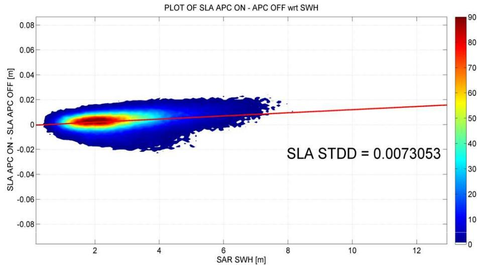
Wave Number SSH spectra with or without APC are equivalent, no major anomaly from the dispersion density plot
