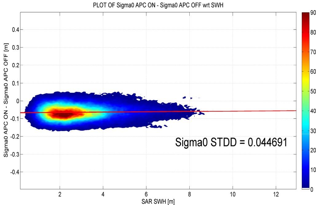
Wave-Number Sigma0 spectrum with APC ON shows lower spectral noise, no major anomaly from the dispersion density plot a part for a static bias (0.07 db)
