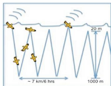
Figure 2. Glider SLOCUM-G1 used in the experiment (left panel) and operating scheme (right panel).
