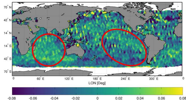
When SRAL operates in OL mode, SARM parameters show a **sensitivity to the echo centering** (epoch). It is visible here when comparing SWH SAR OL to P-LRM or SWH SAR OL to SAR CL during the tandem phase. See Raynal et al., OSTST 2019, effect is about few mm on range and few **cm** on SWH.
