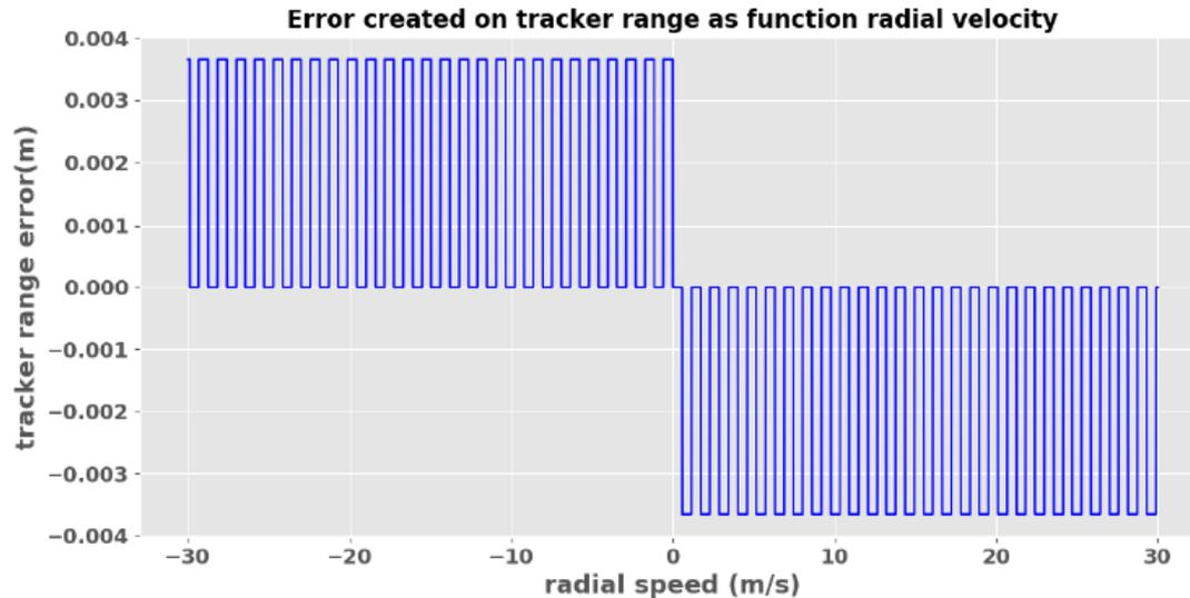
While the impacts created by vertical velocity inaccuracy remain relatively limited in the PLRM estimates (sub-mm bias in range, sub-cm bias in SWH), the **anomaly detected and removed in the PLRM tracker range can create errors of ~3.5mm in the PLRM range.**
