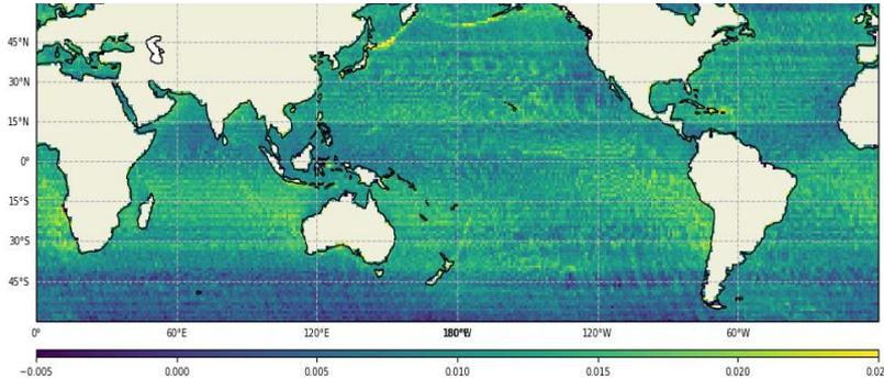
Comparing SARM/PLRM range, **latitudinal effects** are observed. After investigation, J. Aublanc et al. has proved that part of the error comes from **PLRM** processing.
