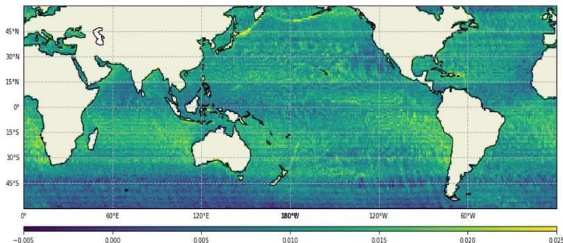
All approximations/anomalies have been corrected within an IPF prototype. Maps of the PLRM range bias between IPF and prototype show as expected latitudinal patterns with  $\sim 3\text{mm}$  amplitude, due to the correction of the tracker anomaly. The impact is predominant wrt the 2 other approximations corrected.
