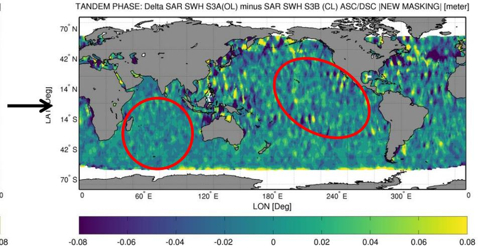
Dynamic masking removed the large-scale patterns correlated to the echo centering.
