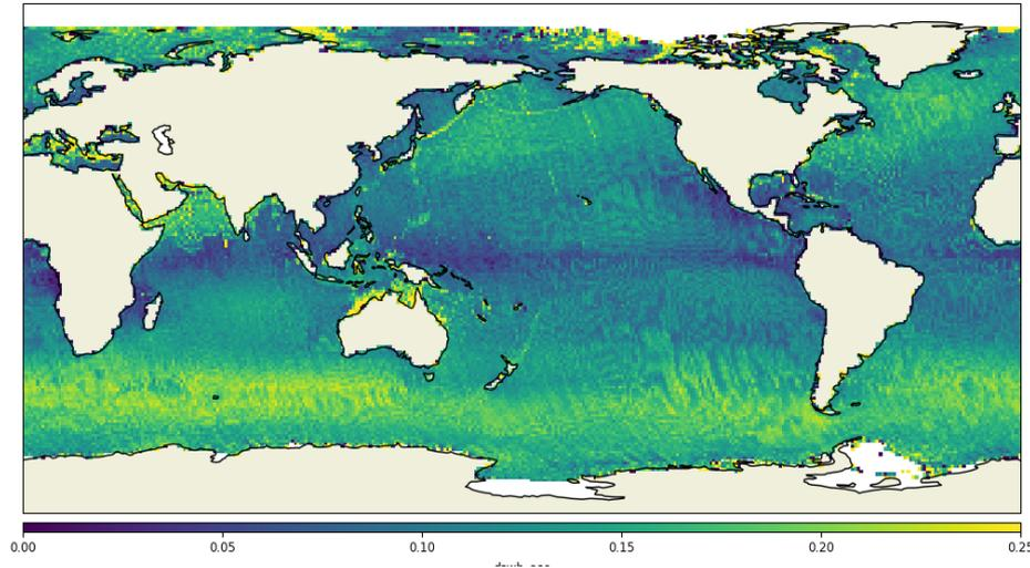
S3B OLTC height – MSS over ascending tracks (meter)
