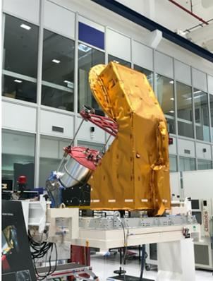
Wave scatterometer using the real aperture concept launched on the 29th of October 2018.
