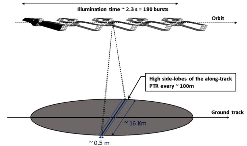
Sentinel-3A FFSAR processing : the altimeter emits 256 times and switch to receive mode. The interleaved mode of Jason-CS/Sentinel-6 (much more continuous) should reduce the high PTR sidelobes
