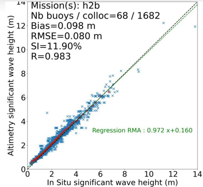
Scatter (blue crosses) and quantile-quantile (red crosses) plot of HaiYang-2B comparison with in-situ measurements [January-June 2020]
