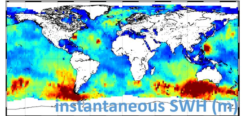
**VAVH\_INST:** weighted average of level-3 available along-track measurements to account for their temporal proximity and spatial interpolation when no measurements
