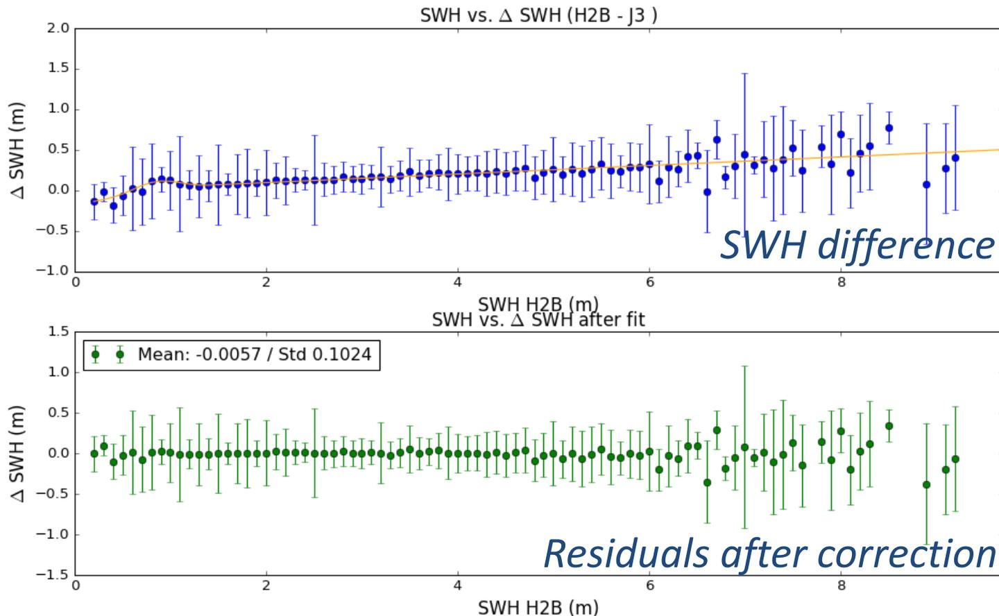
Top: Median of the difference between HaiYang-2B and Jason-3 SWH values at crossover points per 10-cm bin. Error bars represent the standard deviation of the difference inside each bin. The orange curve represents the correction applied. Bottom: Residuals between the median and the fit.
