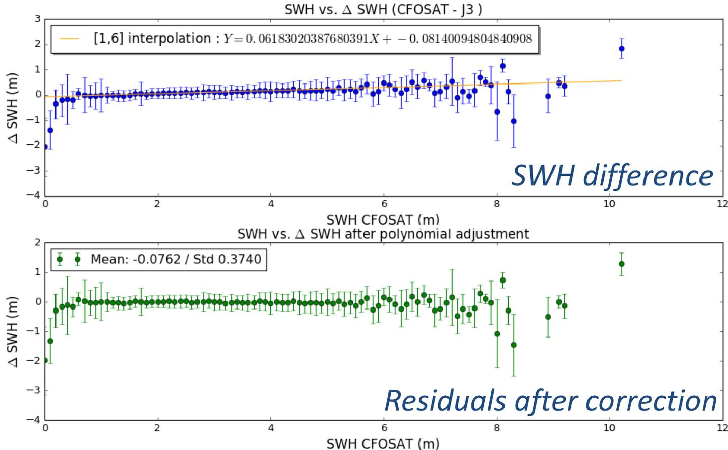
Top: Median of the difference between CFOSAT and Jason-3 SWH values at crossover points per 10-cm bin. Error bars represent the standard deviation of the difference inside each bin. The orange curve represents the linear fit over the [1-6] meter range. Bottom: Residuals between the median and the fit.
