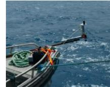
A version of the Cyclopée system (GNSS antenna + acoustic altimeter) installed on N/O ALIS tender
