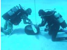
5 pressure sensors deployed in the lagoon (TG1 – TG2 – TG3 – TG4) and outside (TG5). TG1 is under the altimetry crossover points. They will be removed in Autumn 2020.
