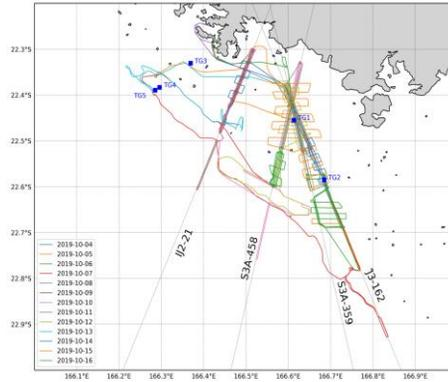
Blue squares correspond to pressure sensors position, grey lines to altimetric tracks. All the colored lines represent ALIS trajectory during the cruise
