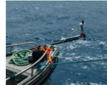
A version of the Cyclopée system (GNSS antenna + acoustic altimeter) installed on N/O ALIS tender
