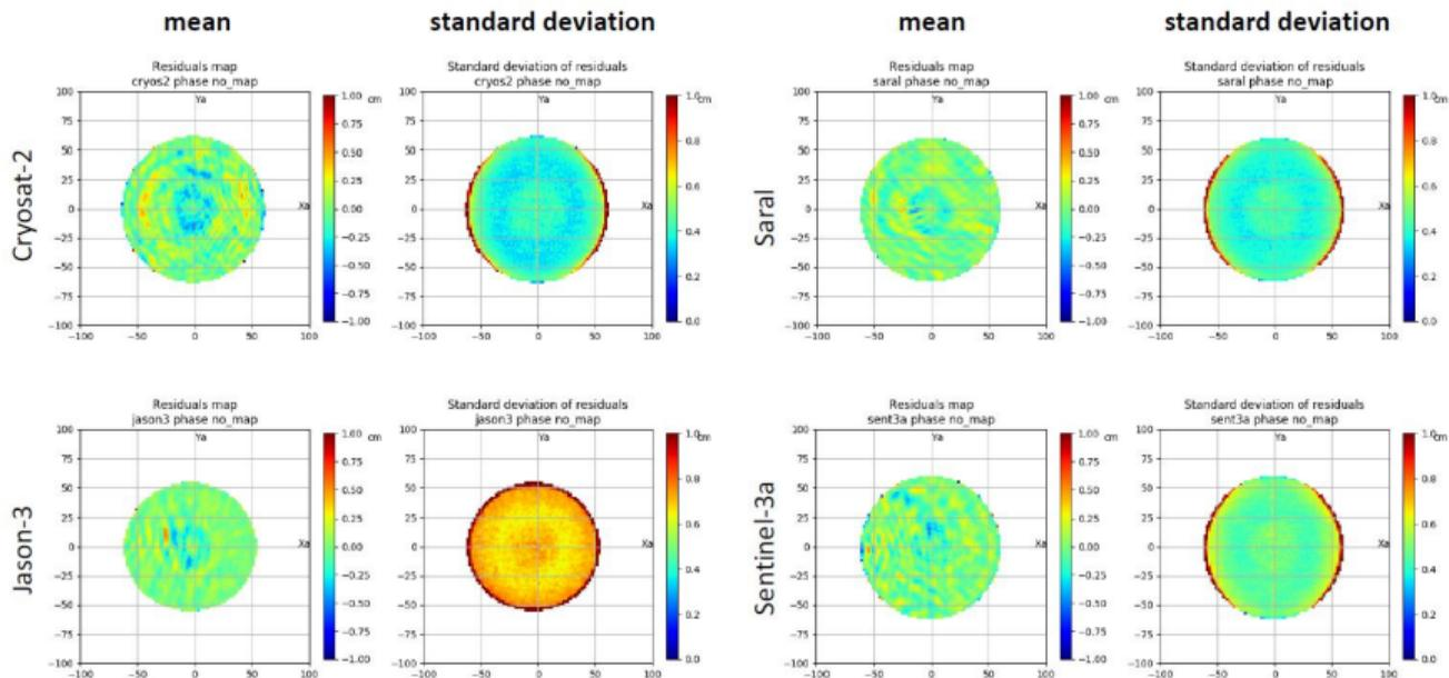
Residual DORIS phase maps (mean/standard deviation) for CryoSat-2, Jason-3, Saral/AltiKa, and Sentinel-3A.
