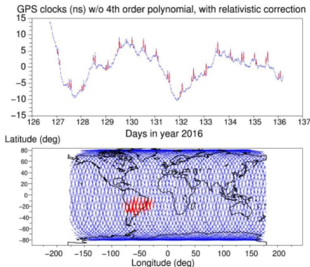
GPS clock and corresponding Sentinel-3A ground tracks (in red for the DORIS USO frequency drifts).
