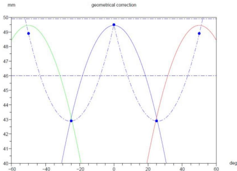
Delays corresponding to the reflexions on the central cube (blue) and two external cubes (green/red) of the Jason LRA assembly as a function of the zenith angle.
