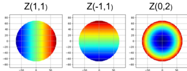
DORIS phase center corrections for CryoSat-2, Jason-3, Saral, Sentinel-3A, and first Zernike modes corresponding to the PCO.
