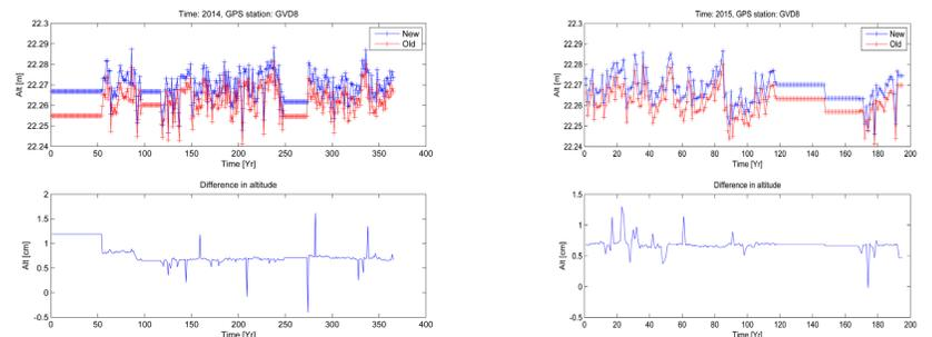
The 2014 (left) and 2015 (right) GVD8 altitude daily solutions of the GIPSY processing using the IGS (red) and "new" (after absolute calibration-blue) derived ANTEX files along with their residuals.
