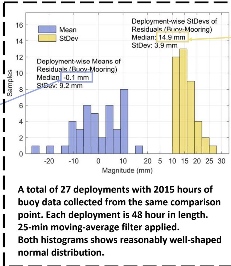
② Median of deployment-wise standard deviations at **~15 mm** (yellow bars) interpreted as the overarching precision of UTas/IMOS Mk-IV GNSS buoy
