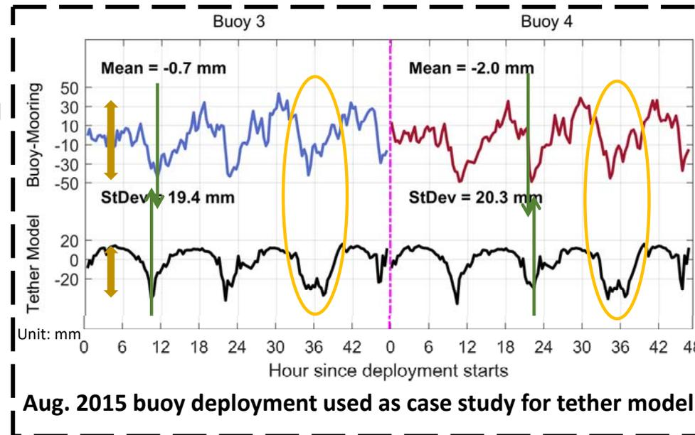
③ We used ACCESS regional wind stress (hourly) and in situ current-meter measurements (20-min) as input to generate the modelled tether tension time series
