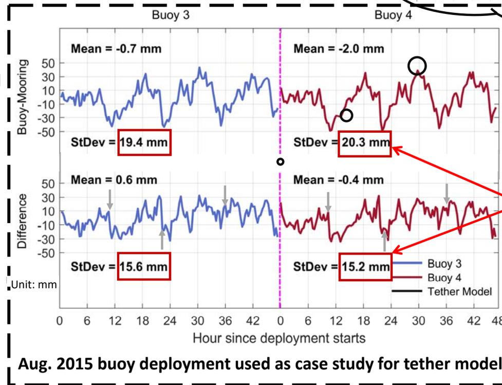
③ Upon removal of the modelled tether tension effect, a **~5 mm reduction** in standard deviation can be observed with obvious **attenuation** of low frequency signals (**semi-diurnal**) and also the mean of the residual brought further to zero.
