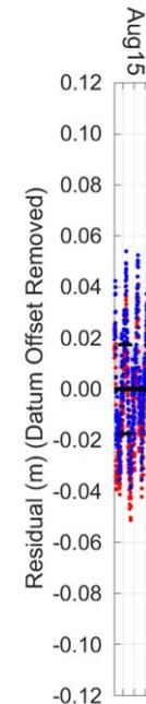
③ Deployments with standard deviation larger than 20 mm, such as in Aug. 2015 deployment, are believed to be affected by external forcing on the tether (wind, waves, currents). Time series of SSH presents dominant semi-diurnal signals.
