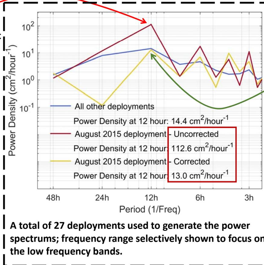
② After applying empirical tether model, **power density** at 12-hour band is **reduced** to the same level as in all other deployments.
