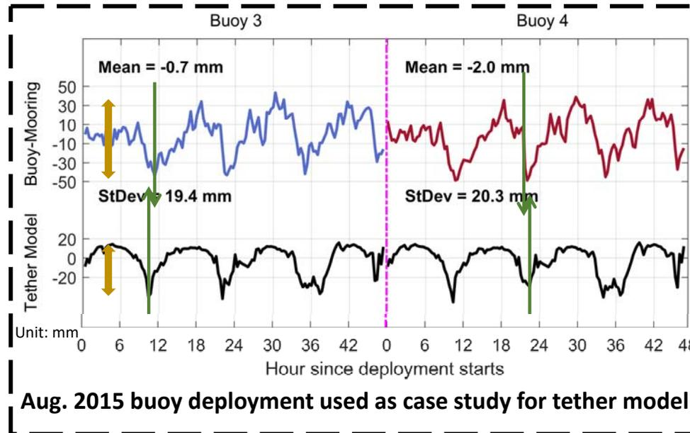
② We used ACCESS regional wind stress (hourly) and in situ current-meter measurements (20-min) as input to generate the modelled tether tension time series
