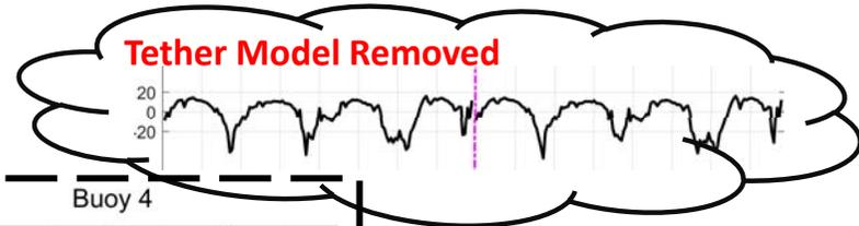
③ Upon removal of the modelled tether tension effect, a **~5 mm reduction** in standard deviation can be observed with obvious **attenuation** of low frequency signals (**semi-diurnal**) and also the mean of the residual brought further to zero.
