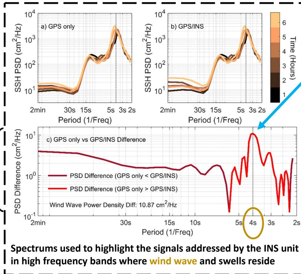
② An over-estimation of the magnitude of wind waves is at  $\sim 11 \text{ cm}^2/\text{Hz}$  for GPS only solutions by failing to address the biases induced by orientation variation of the buoy platform
