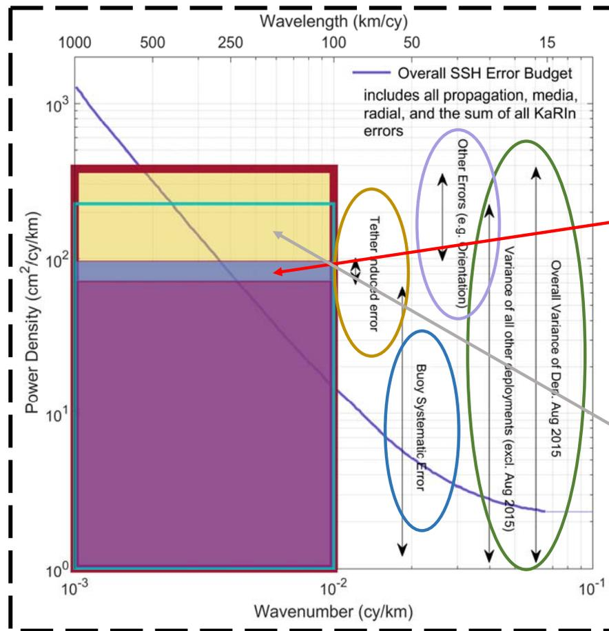
③ Case study of our **empirical tether model** shows a promising energy reduction in low frequency bands associated with a **5 mm** standard deviation **reduction** in the buoy-minus-mooring residual.
