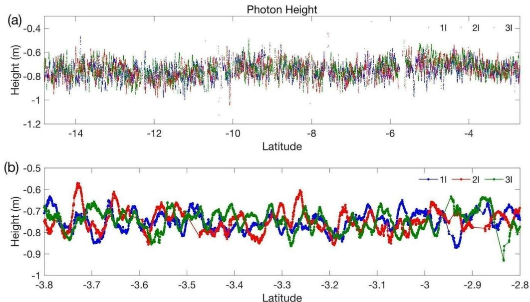
Figure 8. (a) Low-pass filtered (3 km and sampled at 50 m) SLA. Missing data were not included in the filter. (b) a shorter segment of (a). Tracks run almost N-S so  $1^\circ$  corresponds to  $\sim 110$  km along track.
