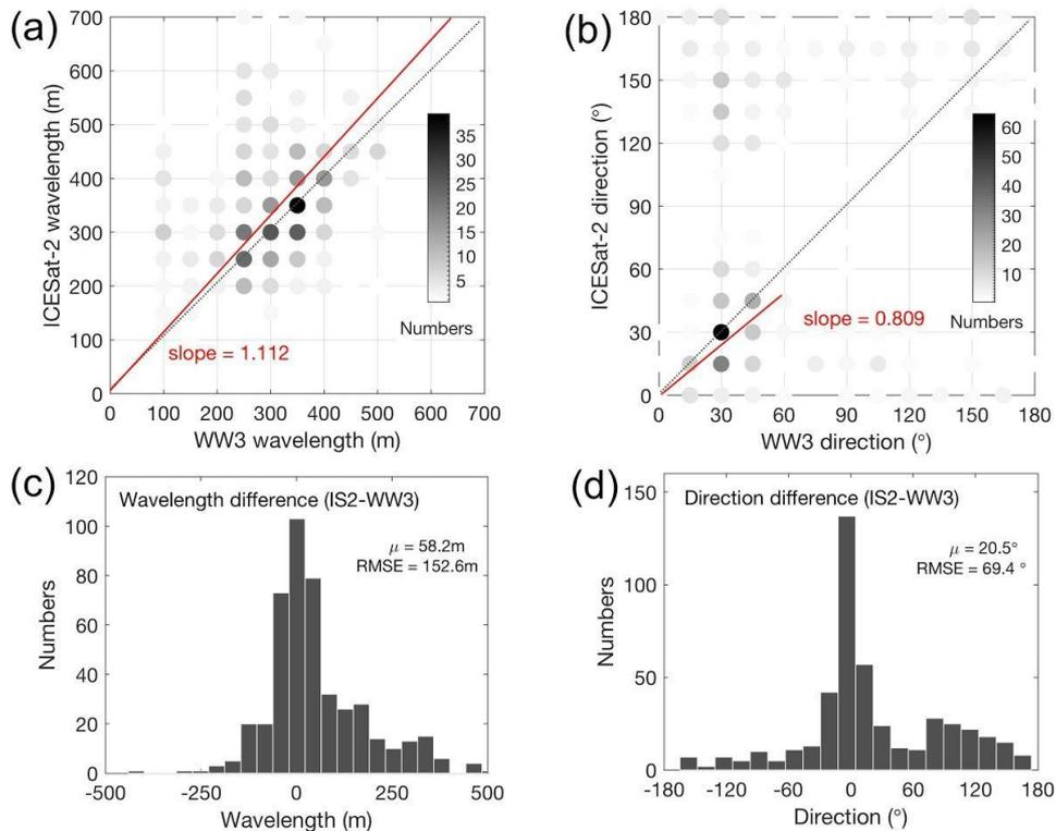
Figure 7. Joint probability histograms for wavelength (a) and wave directions (b) of WAVEWATCH III (WW3) predictions and ICESat-2 (IS2) reconstructions. The black dotted line is the 1:1 relationship and the red line is the best fitted slope. Histogram of (c) wavelength and (d) direction differences between IS2 reconstructions and WW3 predictions.
