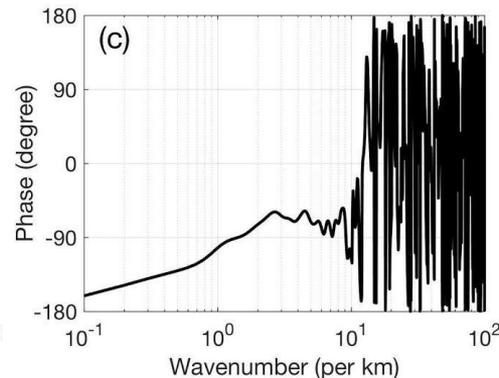
Figure 6. (a) a small segment of ICESat-2 photon height data w.r.t WGS 84. (ground track: 0326, cycle: 01). The strong and weak beams are separated by 90 m and both are low-pass filtered at 30 m. (b) Coherence and (c) phase between beams 1l and 1r. Coherence peaks around 465 m and the corresponding phase shift is  $-70.3^\circ$ . The 95% and 99% CL are labeled.
