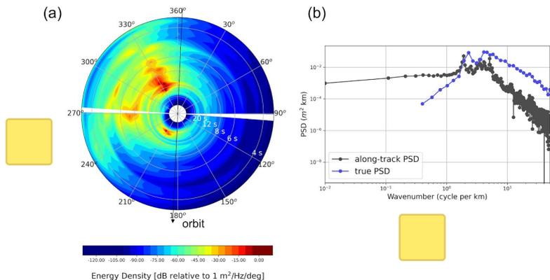
Figure 9. (a) Directional spectrum from CDIP station Point Reyes at time: 2019-09-29, 19:00 UTC. Energy density is in dB so as to show a large range of energy levels. The directional spectrum was computed using the maximum entropy method (Lygre et al., 1986). ICESat-2 orbit inclination is  $92^\circ$  and here we show a synthetic descending track. (b) grey: along-track PSD; blue: true PSD. Both are derived from the directional spectrum in (a).
