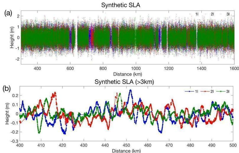
Figure 10. (a) Synthetic SLA using CDIP directional spectrum in Figure 8 (a) and the positions of ICESat-2 track (ground track: 0394, cycle: 02). The SWH is 2.8m for all three beams. (b) 3km low-pass filtered synthetic SLA for a 100-km segment.
