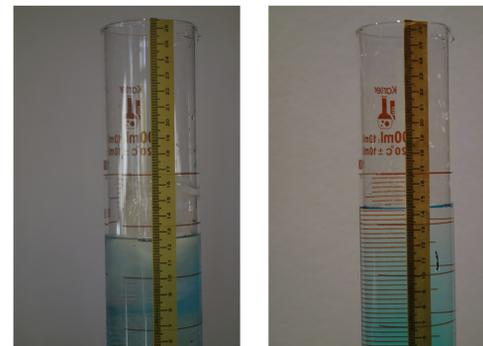
**Fig. 4.** The initial experiment was performed starting with 600 ml of salt solution in the graduated cylinder and a reference height of 3.3 cm on the metric ruler. A total of 333 grams of ice was added, increasing the water level to 12.5 cm (left). Melting overnight raised the water level to 14.4 cm (right).
