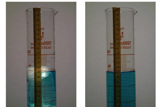
**Fig. 5.** The experiment was repeated, this time using distilled water instead of the saturated salt solution. A total of 290 grams of ice was added to the graduated cylinder, increasing water level to 13.9 cm (left). Melting overnight resulted in no change in the water level from the initial height of 13.9 cm (right).
