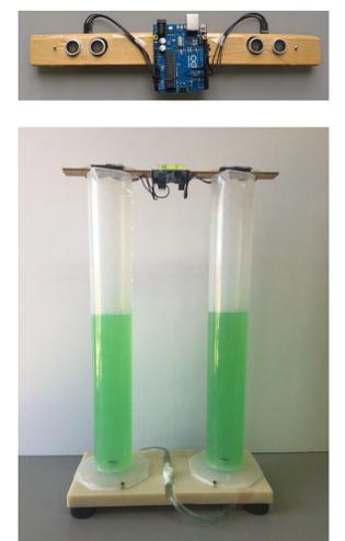
**Fig. 6.** Double altimeter/cylinder configuration.
