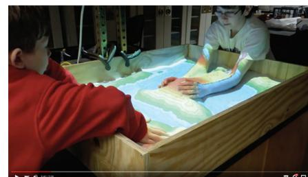
measuring/imaging ocean topography along a swath 120-km wide. We are exploring the use of an augmented reality sandbox as a demonstration tool for this technology. An example is shown to the left.
