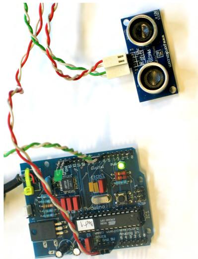
**Fig. 1:** Model altimeter constructed from an Arduino mini controller and an ultrasonic rangefinder.
