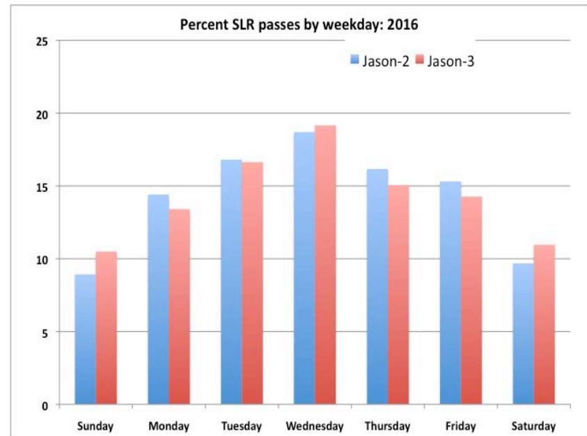
**SLR Tracking for J2, J3 (2016) similar to that provided for earlier missions; Amount of data was similar for both satellites due to interleaving during the satellite passes.**
