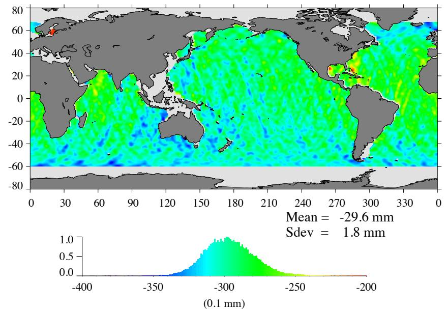
**Std. Deviation of SSH differences is reduced from 3.4 mm to 1.8 mm;
