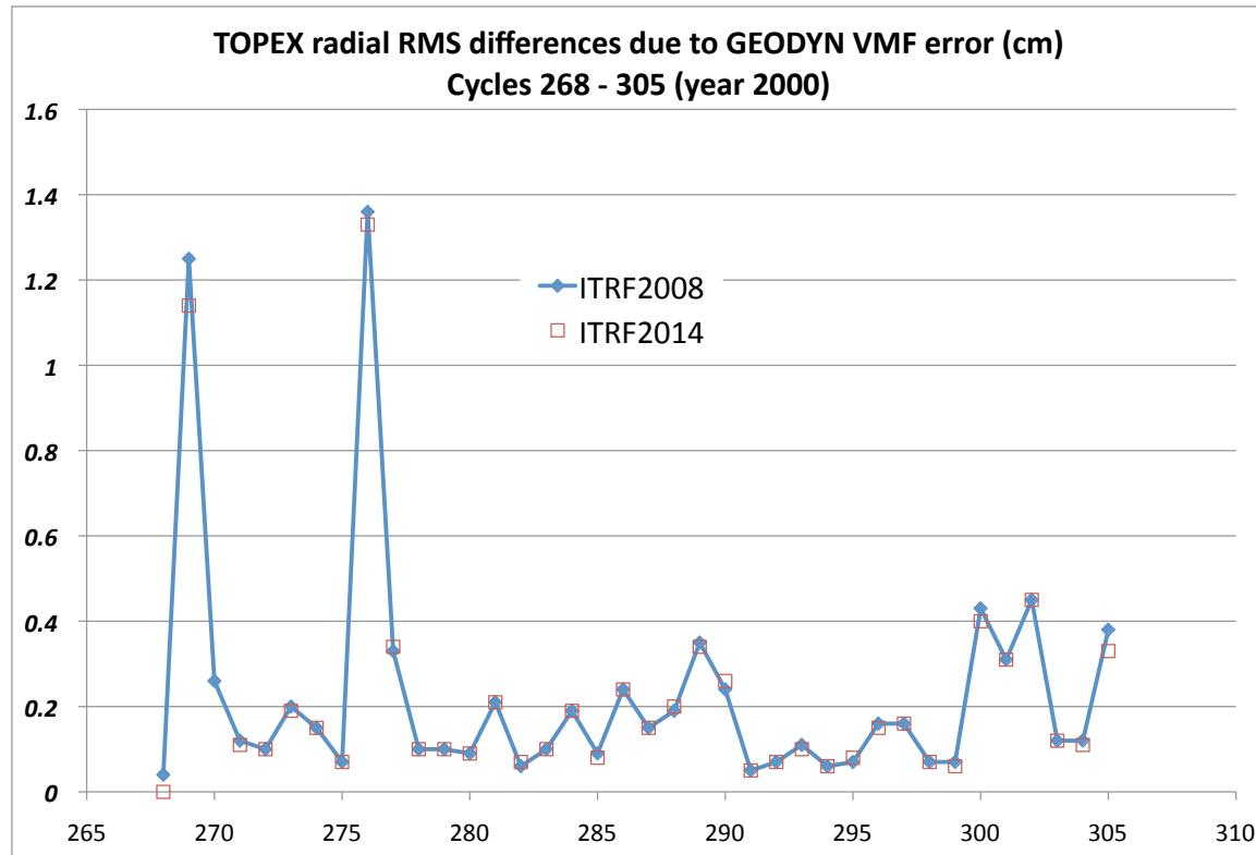
The original TP orbits for the year 2000 (TP cycles 268-305) were affected by an error in the implementation of the Vienna Mapping Function1, used to compute troposphere refraction for the DORIS data. The corrected orbits were redelivered to the NASA CDDIS. The effect is < 2mm radial RMS for most cycles, except cycles 269 & 276, where sparser SLR tracking meant the error was more consequential.
