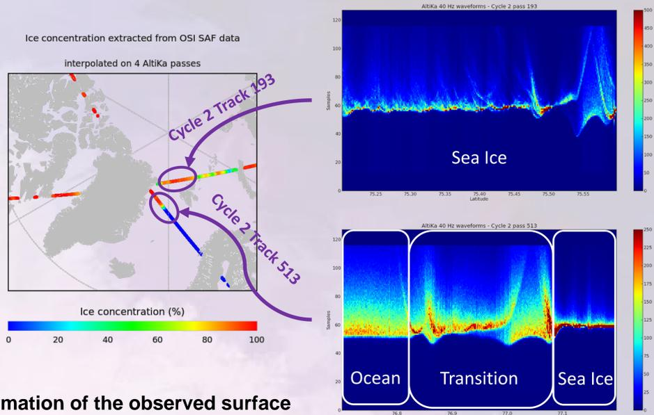
→ A waveform classification can provide important information of the observed surface
