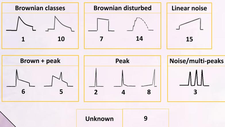
In the frame of the **PEACHI** project supported by CNES, a waveform classification was developed to distinguish different shapes of AltiKa 40 Hz waveforms over all surfaces (ocean, coastal areas, sea ice, continental ice and hydrology) but with a specific focus on sea ice. The classification algorithm is based on a **neural network algorithm** which attributes to an AltiKa echo one of the twelve defined classes from the following parameters:
