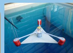
Figure 5 : GNSS equipped buoy
