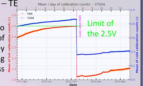
On the **22th october 2013**, a new value of the offset voltage has been uploaded in the on-board database which allowed to retrieve a correct dynamic of the gain.
