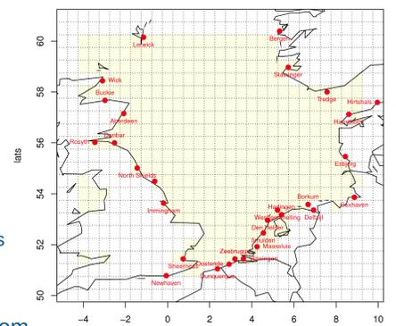
Fig. 3: Positions of used tide gauge data, area covered by altimetry (shaded) and altimetry grid.
