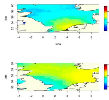
Fig. 8: Linear trend in [mm/year] for 1993-2012 by altimetry (above) and from the reconstruction (below) and from a reconstruction based on GPS corrected tide gauges (right).
