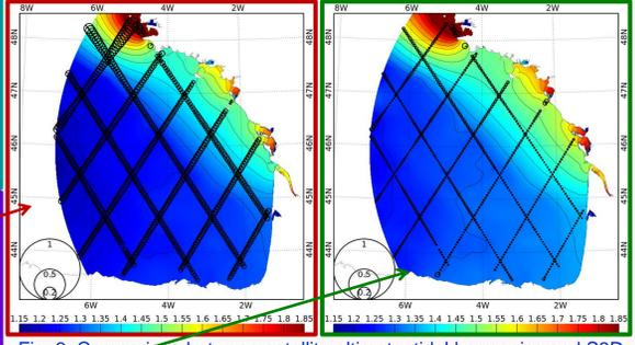
Fig. 3: Comparison between satellite altimetry tidal harmonics and S3D for M2. The circle size is proportional to the complex error.
