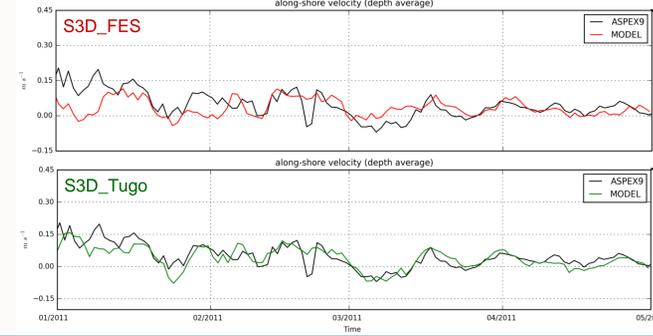
Fig. 5: Daily means of 2D current velocities, projected on the along-shore and the cross-shore axes (left) and ADCP locations from Le Boyer et al. (2013) (right)
