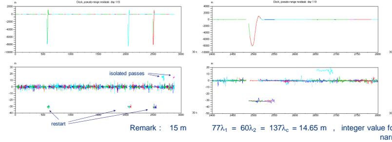
The biased pseudorange measurement are used for the widelane solution.
