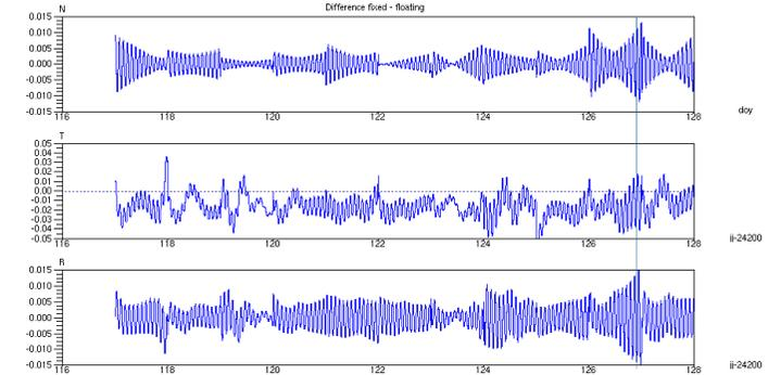
The along track bias is now correct. The radial effect is ~5 mm rms between floating and fixed cases (dynamic orbits)
