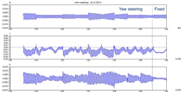
Due to drifts in the phase measurement : the pseudo-range clock is different from the phase clock (200.0.02 case)
