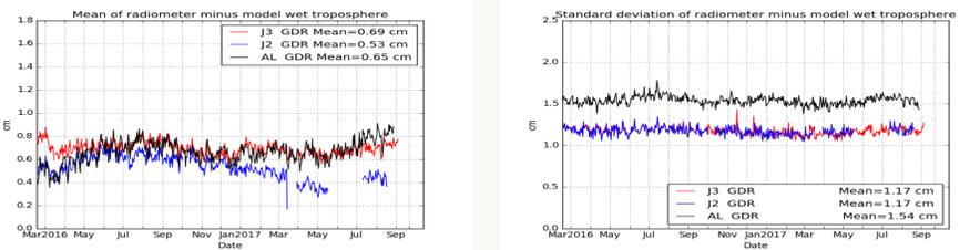
Radiometer minus model wet tropospheric correction compared to other missions
