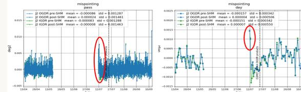
mispointing was slightly increased just after SHM, but only on the first passes: it has been nominal since new instrumental parameters LTM have been applied.
