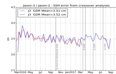
Performance at crossovers: left: map of mean SSH differences (cycle 000 to 504). right: SSH error deduced from SSH crossovers (using radiometer data, with selection on |latitudes| < 50°, bathy < -1000m, oceanic variability < 20 cm)
