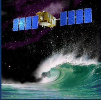
After almost 9 years in orbit as a precise altimeter mission on two different repeat ground tracks, Jason-2 had early this year an interruption of its science mission from 17th May to early July 2017. In the following, it was moved to a long-repeat ground track. Though this orbit is less interesting for the tandem mission with Jason-3 to observe mesoscale ocean signals, the mission can still provide valuable and useful data for several applications.
