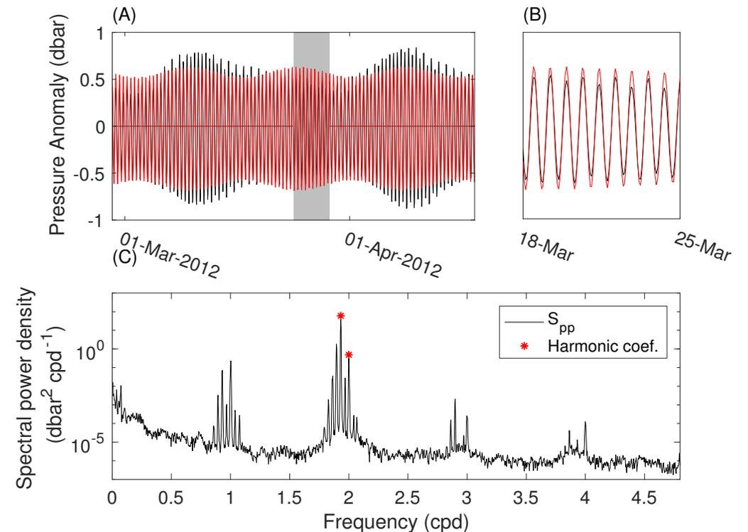
Harmonic analysis of a bottom pressure time series (A, with B as the zoomed in gray segment), fit to two tidal frequencies. With substantial energy at many constituent frequencies (C), much variance remains unmodeled.
