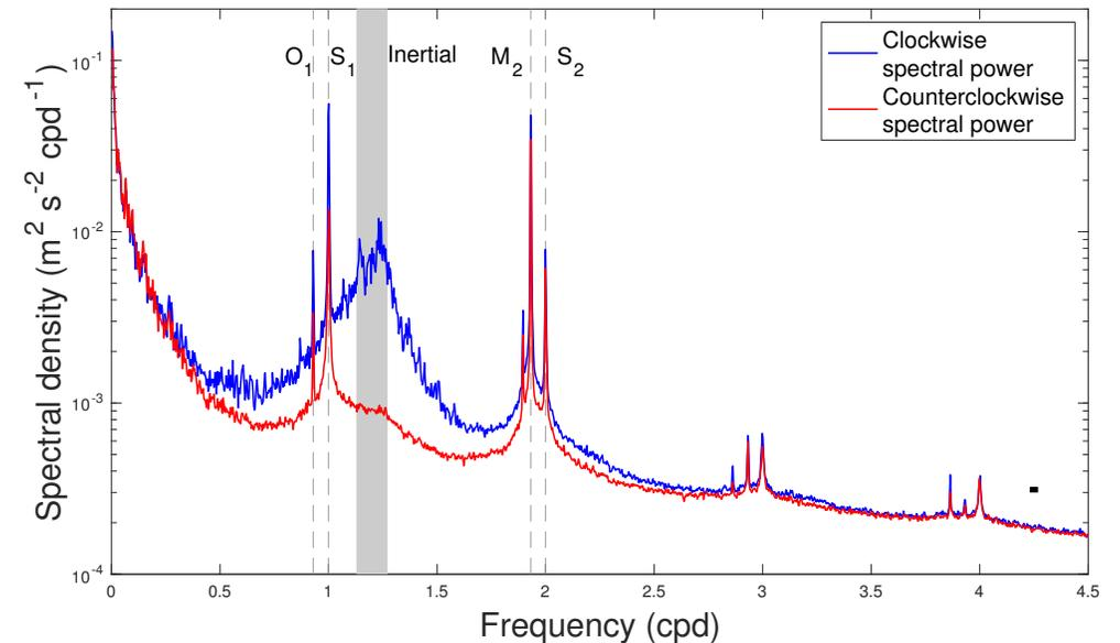
Rotary spectrum of surface currents observed by high-frequency radar. This is an example of a tidally-driven record with substantial non-stationary energy (broad cusps) and an energetic red background.
