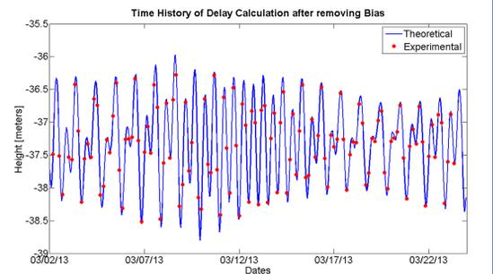
**Figure 6:** This figure shows time history of experimental delay after removing the mean of the offset. This is plotted along with the expected delay computed from the tide gauge SSH values. It is noted that both the plots follow each other closely. The standard deviation was found to be 0.18 meters.
