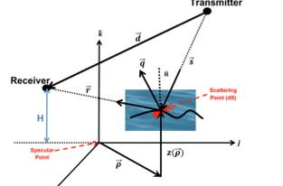
**Figure 3:** The geometry of the problem is shown in this figure. A direct signal from the satellite and a reflected signal from the ocean surface is recorded by the receiver.
