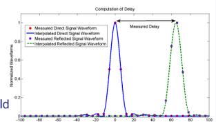
**Figure 4:** This figure shows an example of the path delay between the direct and reflected waveform.
