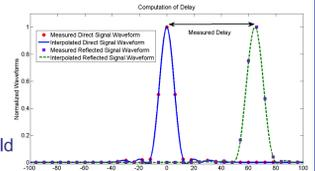
**Figure 4:** This figure shows an example of the path delay between the direct and reflected waveform.
