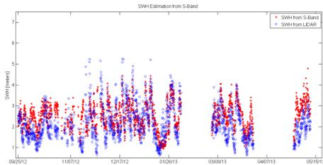
**Figure 8:** This figure shows a time series of SWH estimation from the S-band. The standard deviation of the error in estimation was 0.44 m.
