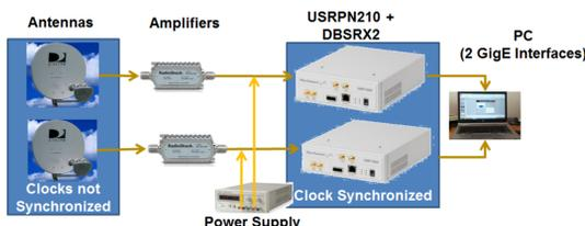
**Figure 2:** This figure describes Ku-band receivers. The signals captured by the antennas are downconverted, digitized, and sampled by Universal Software Radio Peripherals (USRPs), which then transfers data to a computer to be stored.
