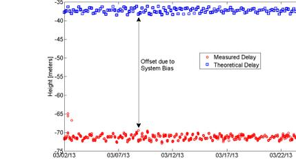
**Figure 5:** This figure shows the offset between the theoretical delay and experimentally computed delay due to system bias. The mean of the offset was found to be 33.86 meters.
