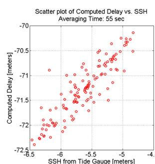
**Figure 7:** This figure shows a scatter plot of computed delays vs. the SSH measured by the tide gauge located at Platform Harvest. The correlation coefficient was found to be 0.90.
