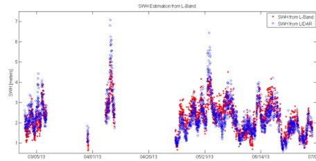
**Figure 9:** This figure shows a time series of SWH estimation from the L-band. The standard deviation of the error in estimation was 0.40 m.
