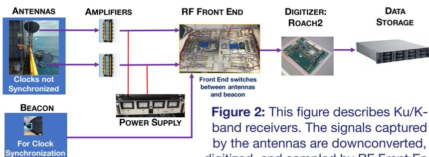
**Figure 2:** This figure describes Ku/K-band receivers. The signals captured by the antennas are downconverted, digitized, and sampled by RF Front End and CASPER ROACH2 digitizer, and transferred to hard drives for storage.
