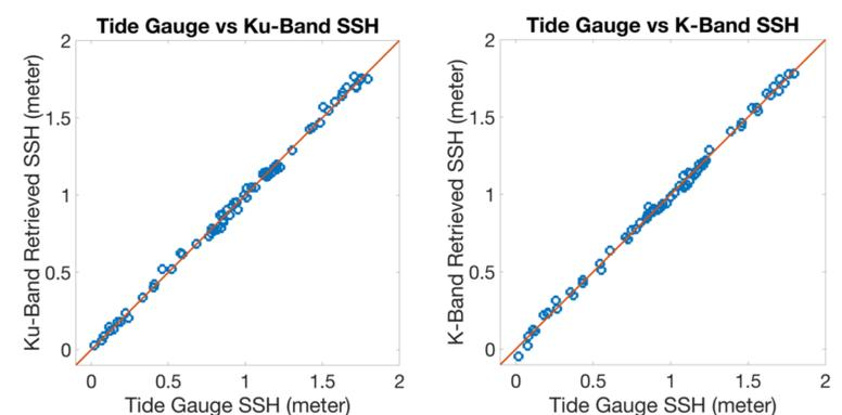
**Figure 4:** The figure shows scatter plot of retrieved SSH from Ku-band (left) and K-band (right) LHCP data and SSH from tide gauge. The error in retrieval of Ku-band and K-band is 2.69 cm and 2.61 cm, respectively.
