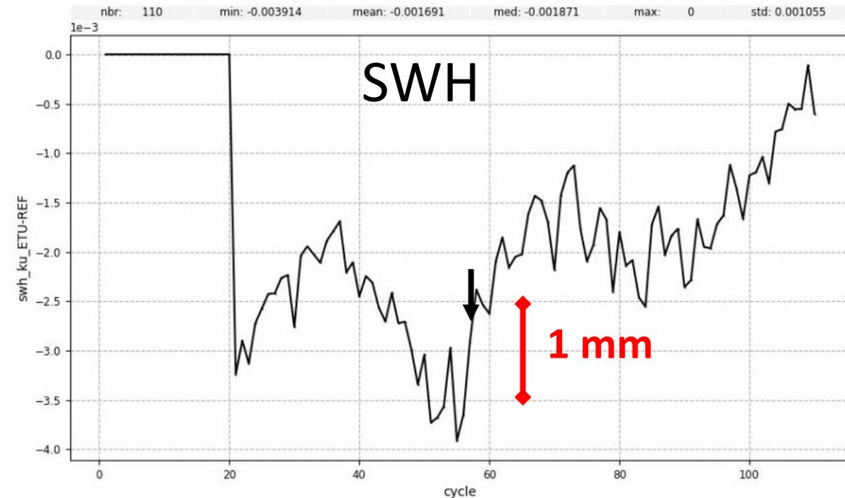
Cycle 21 LUTs have been applied from cycle 21 but should be applied from cycle 4 (instrumental restart at cycle 3 track 181). Very weak impact on the SWH can be observed with variations of one/two millimeters
