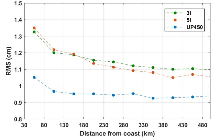
↑ RMS of the WTC differences between SIMWR and 3I, 5I and UP4S0 function of distance from coast.
