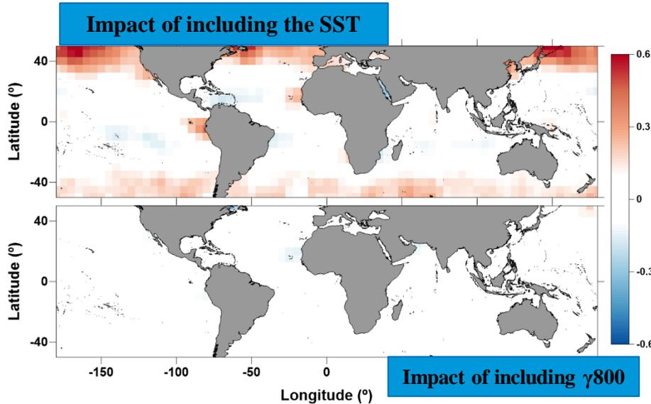
↑ RMS decrease (cm) when compared with SIMWR for UP3S0-UP4S0 (top panel) and UP4S0-UP5S0 (bottom panel).
