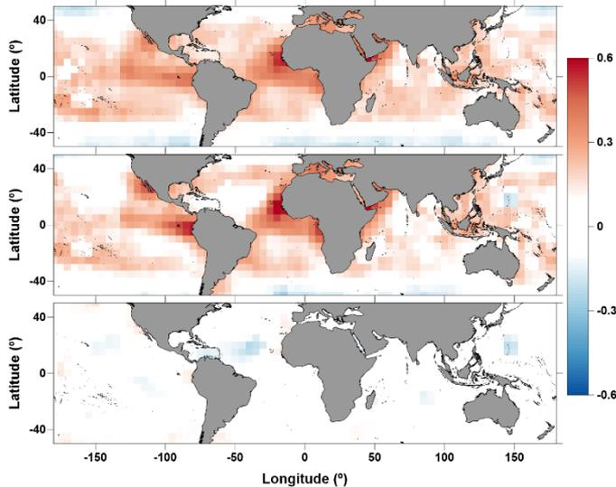
↑ RMS decrease (cm) when compared with SIMWR for 3I-UP3S0 (top panel), 3I-UP3WS (middle panel) and UP3S0-UP3WS (bottom panel). Red colour indicates decrease in the RMS.
