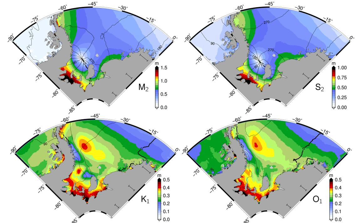
**Figure 9:** The four largest tides mapped from CryoSat-2 data. The amplitude is shown with the color scale, and phase lines are shown in 30° increments.
