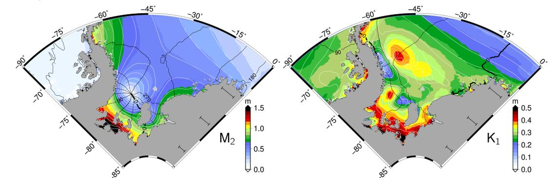
**Figure 10:** Comparison of the  $M_2$  and  $K_1$  tides from CryoSat-2 (color) versus CATS8a (white contours).
