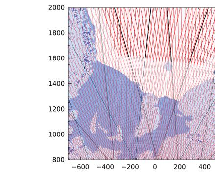
**Figure 2:** CryoSat-2 ground tracks during a 30-day period (polar stereographic projection with easting and northing indicated in units of km). Black lines indicate tracks within a 3-day pseudo-subcycle.
