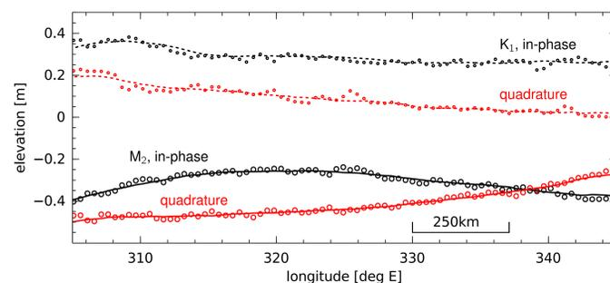
**Figure 6:** Tidal harmonic constants computed from CryoSat-2 data along a section at 70°S. Analysis of data within large spatial bins (lines) is needed to sample tidal phases uniformly, as compared with analysis of data within small bins (dots).
