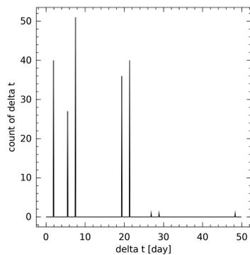
**Figure 3:** Histogram of sample interval for CryoSat-2 data within a 30 km-diameter disc at 70°S. Samples near  $\Delta t = 2$  days and  $\Delta t = 29$  days are associated with pseudo-subcycles. Samples near  $\Delta t = 6$  days and  $\Delta t = 20$  days are associated with intersecting ascending and descending tracks.
