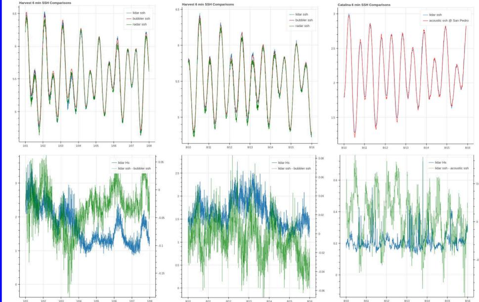
Top row: Example time series of lidar SSH measurements taken at Harvest Platform (1<sup>st</sup> and 2<sup>nd</sup> columns) and Catalina (3<sup>rd</sup> column) and compared with the collocated traditional bubbler tide gauge and radar tide gauge SSH measurements.
