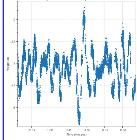
Top Right: Example raw 500Hz lidar range measurements from July 3, 2017, measured at the Catalina site showing a much calmer wave state in Fisherman's Cove. Note the lidar at Catalina shows evidence of the discrete range bins and penetration below the water surface.
