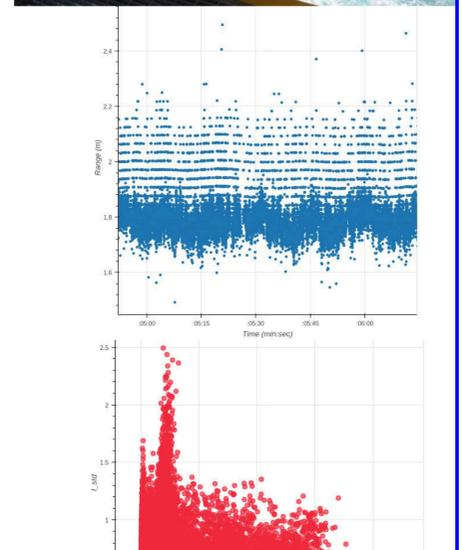
Below: Example raw 500Hz lidar range measurements from July 3, 2017, measured at Harvest Platform showing individual wind waves and swell. Note the lidar (like the altimeter) only reflects from specular facets on the surface and therefore has periods of missing returns.
