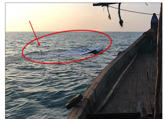
Fig. 2: Our observational device off the coast of Cox's Bazaar, Bangladesh, in November 2014. The CalNaGeo towed raft is highlighted in red. The arrow points to the GNSS antenna.
