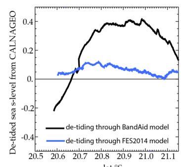
Fig. 9: CalNaGeo SSH residuals obtained after removing BandAid tidal heights (black) and FES2014 tidal heights (blue). BandAid model advanced by 20min was considered.
