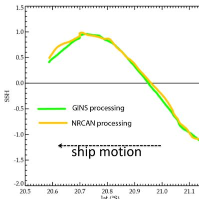
Fig. 7: SSH measurements from CalNaGeo after a 15min filtering (equiv. to ~2.5km), along the southward transect seen on Fig. 1. Reference is CNES-CLS2011 MSS.
