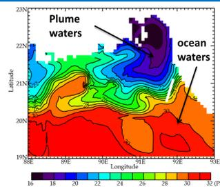
Fig. 4: Sea surface salinity on 9/11/2014. CalNaGeo transect is shown in white, right on the salinity front separating the river plume and open ocean waters.
