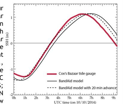
Fig. 8: SSH recorded by Cox's Bazaar tide gauge (in red) and simulated by Band-Aid model (black) during the same period as Fig. 7.
