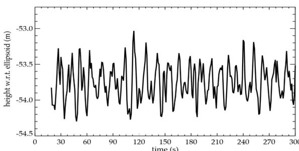
Fig. 6: Raw SSH measurements from CALNAGEO over 10min on 10/10/2014. Reference is GRS80 ellipsoid.
